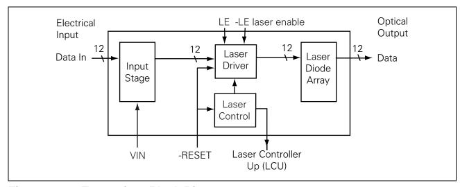
Figure 2 Transmitter Block Diagram
