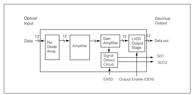
Figure 3 Receiver Block Diagram
