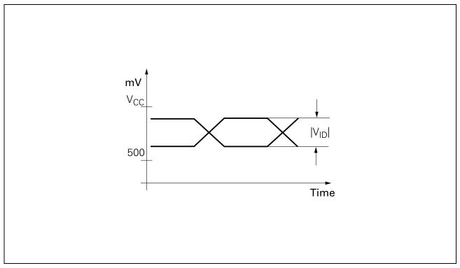
Figure 5 Input Level Diagram
