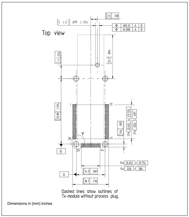
Figure 11 Recommended Circuit Board Layout: Transmitter
