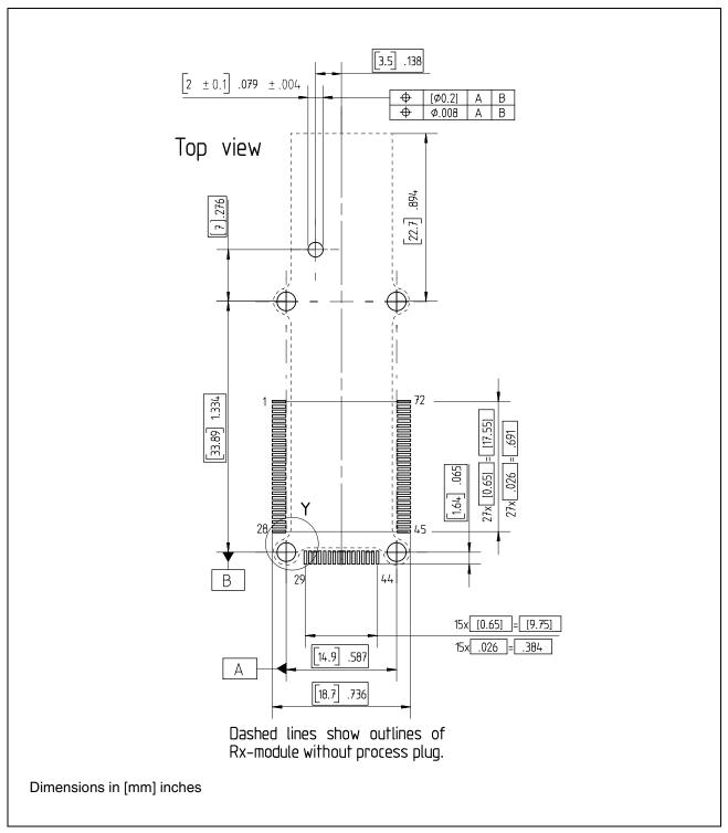
Figure 12 Recommended Circuit Board Layout: Receiver
